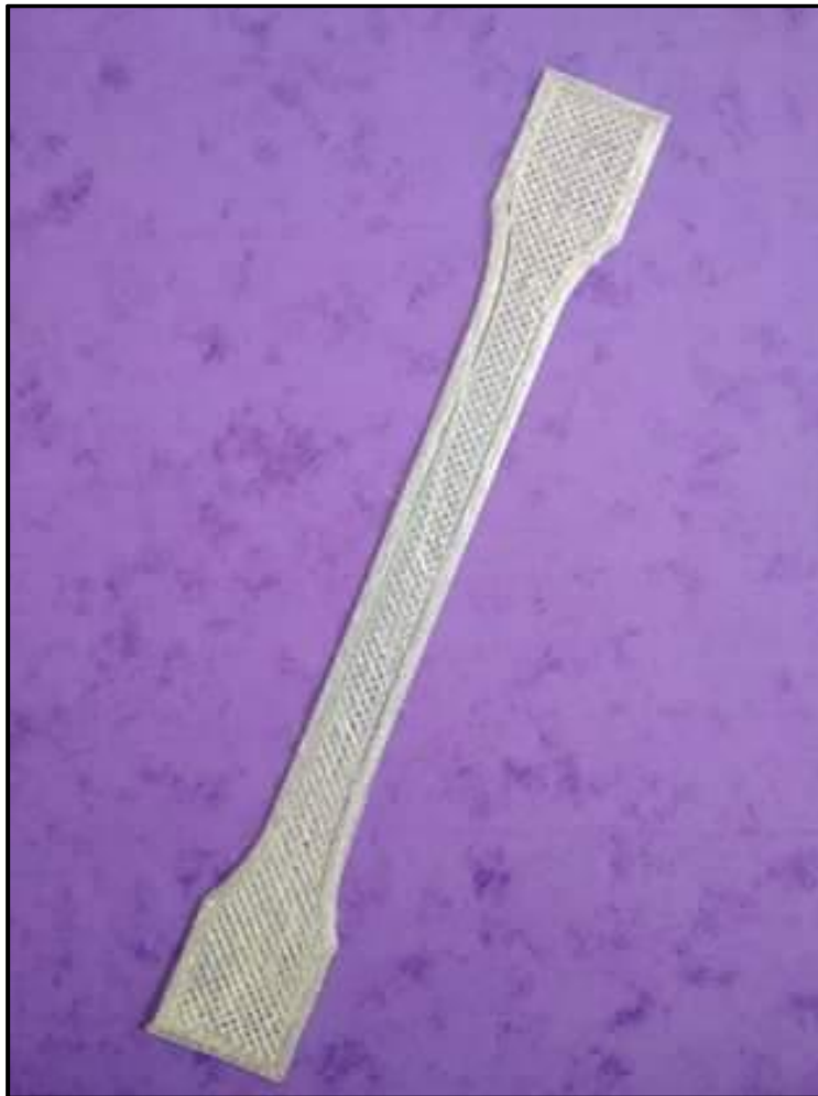
Figure 46. First 3D printed piece with the extruded Pellethane 2102-90A filaments
