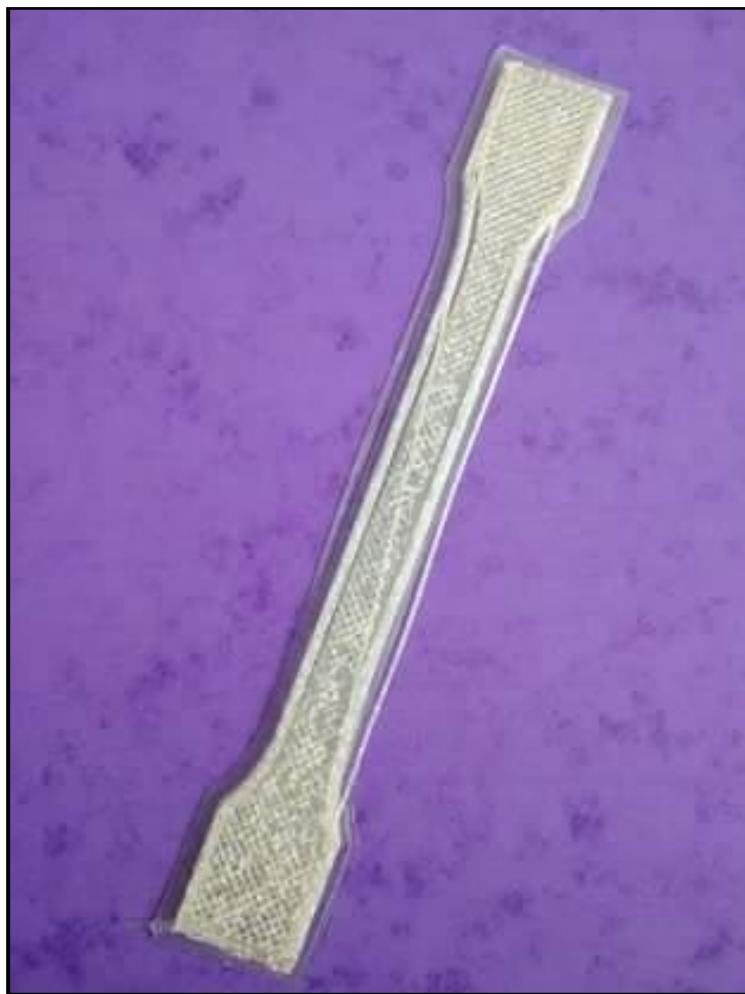
Figure 47. Second 3D printed piece with the extruded Pellethane 2102-90A filaments
