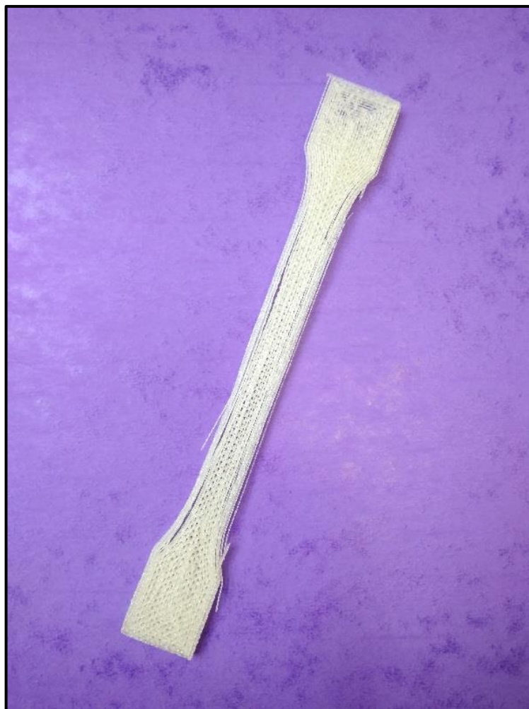
Figure 48. Third 3D printed piece with the extruded Pellethane 2102-90A filaments
