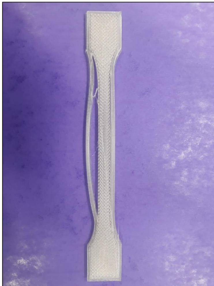
Figure 45. 3D printed piece with the extruded Pellethane 2102-65D filaments
