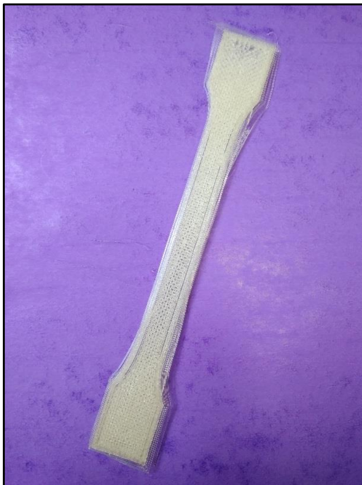
Figure 49. Fourth 3D printed piece with the extruded Pellethane 2102-90A filaments
