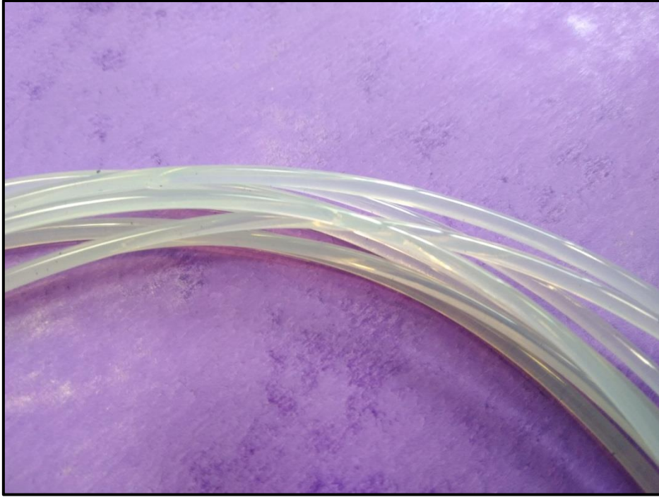
Figure 44. Detail of the Pellethane 2102-90A filament (E2P90A)
