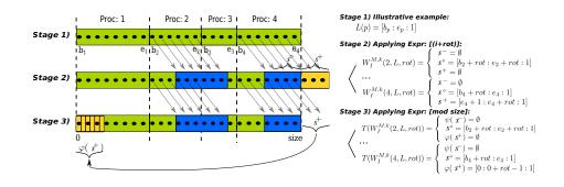
**Figure 9.3:** Communication structures calculation. Using the read data-access expression inside the parallel computation of the illustrative example to build the functions that calculate the working input indexes set ( $W_I$ ), for the data structure M, for the processes 2 and 4. This example uses contiguous rectangular shapes, an irregular data partition policy, and depicts the particular case of rot = 3, for a domain with  $|M_0| = 25$ .
