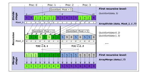
**Figure 10.6:** Sequence of operations performed in the QuickSort algorithm in a distributedmemory system using the *ArrayDivide* and *ArrayMerge* operators. *T* function assigns to each group array a number of processes that is proportional to the size of the group array.
