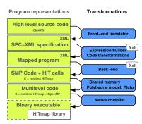
Figure 8.5: Structure of the Trasgo transformation framework.
