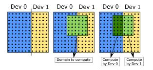
Figure 5.2: Calculating the domains to compute for each device.
