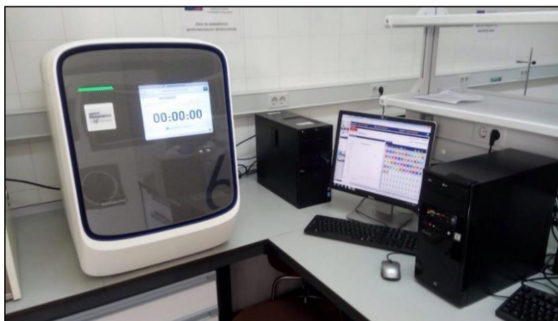
Figure 5. QuantStudio 6 Flex Real-Time PCR System used for the real-time PCR reactions. Photo credit: Pablo Martínez Álvarez.
