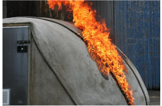
Photography 16. Concrete Canvas pneumatic shelter. Fire behaviour. Source: https://www.flickr.com/photos/_concretecanvas/sets/72157638403394195/
