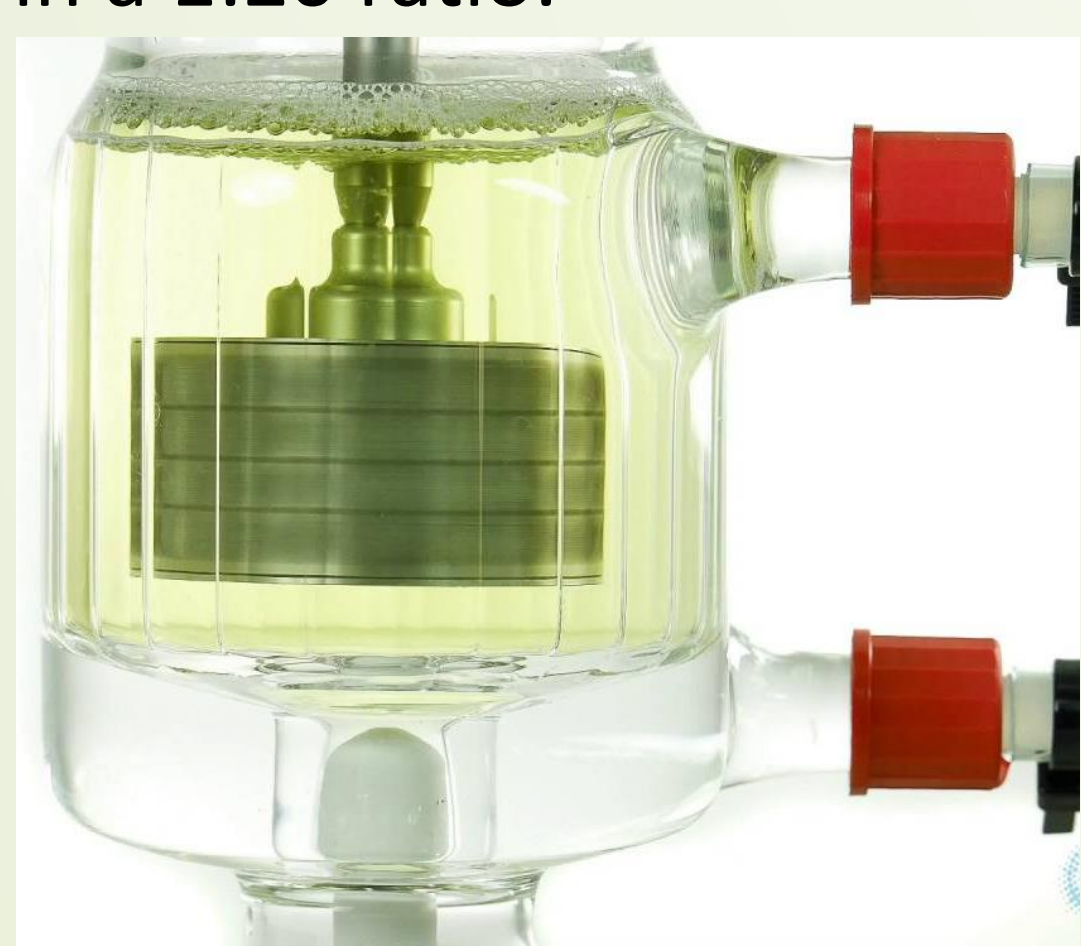
Figure 4: Rotating bed Reactor
