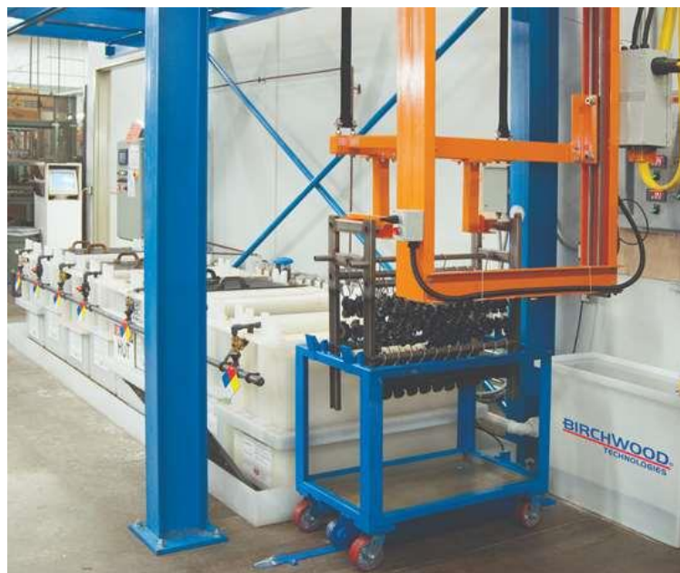
Figura 10. Sistema de óxido negro “CNC Tru Temp”. https://www.birchwoodtechnologies.com/blackening_time_reduced_using_automated_tru_temp_system/
