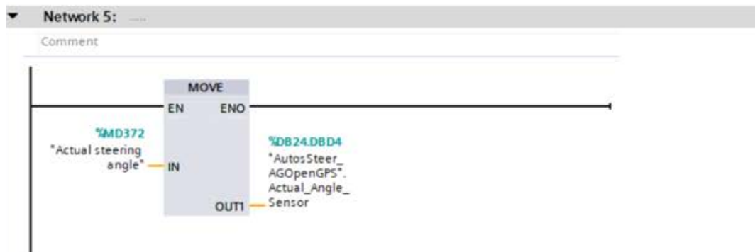
Figure 64. Sending the actual angle's value to a DataBlock .
