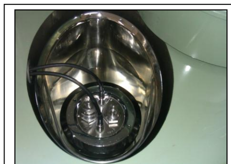
Fig. 8. Bomb of combustion with the electrodes and the water vessel inside the calorimeter.
