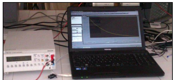
Fig. 5. Multimeter with a Pt-100 and a computer for monitoring the temperature.
