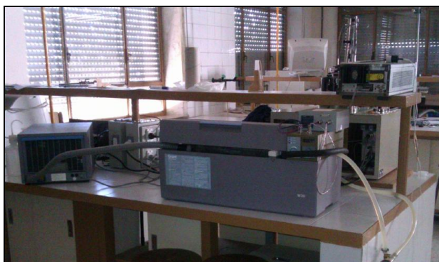
Fig. 6 and 7. The refrigerated immersion cooler, the heated water bath and the calorimeter, respectively
