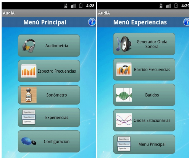
Figure 3. Two screenshots of two of the menus in one of our applications on sound measurements. As this application was developed in order to check if smartphones could be used as reliable laboratory devices, an important point in its development was the inclusion of a calibration of its microphone and speaker.
