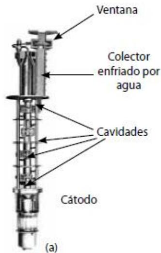
**Figura 5. 8 Klystron [6]**
