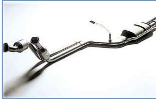
Figure 3.18 – Close-coupled catalytic converters, with underfloor catalyst and oxygen sensor.
