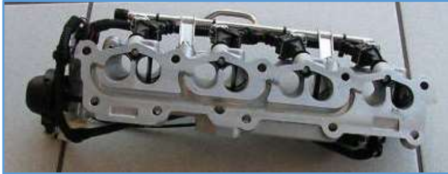
Figure 3.13 – Opel port deactivation system.
