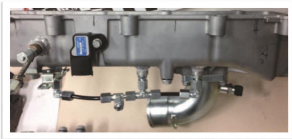
Figure 36. Sampling points for measurements on the intake manifold
