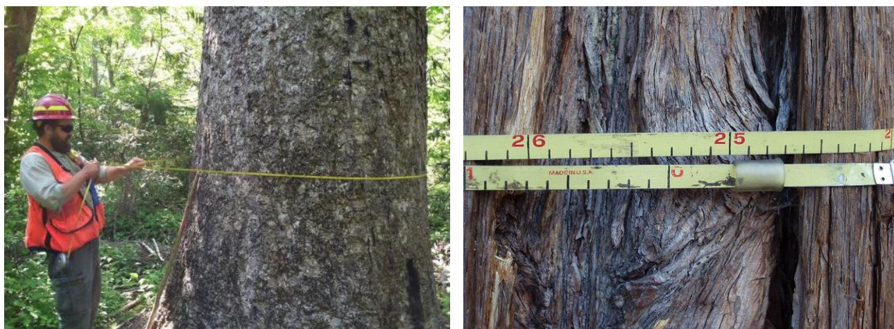
Figure 6. Measurement of the diameter, using a diameter tape wrapped around the main stem of the tree
