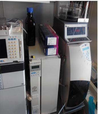
Figure 03. Size-Exclusion Chromatography (SEC) equipment. Åbo Akademi University (ÅA). Laboratoy of Wood and Paper Chemistry.
