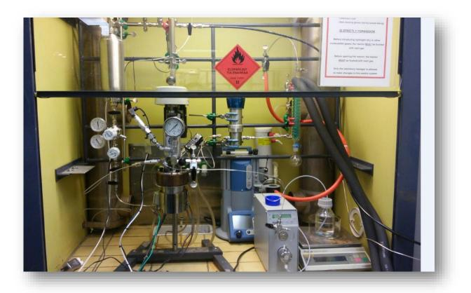
Figure 10. Experimental set up used in copolymerization reactions. Åbo Akademi University (ÅA). Laboratory of Industrial Chemistry and Reaction Engineering.
