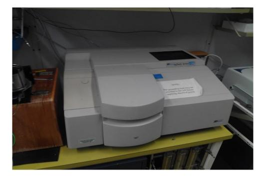
Figure 02. Fourier Transform Infrared (FTIR) equipment. Åbo Akademi University (ÅA). Laboratory of Industrial Chemistry and Reaction Engineering.
