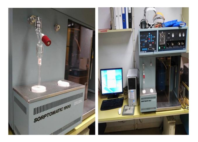
Figure 08. Physisorption equipment. Åbo Akademi University (ÅA). Laboratory of Industrial Chemistry and Reaction Engineering.
