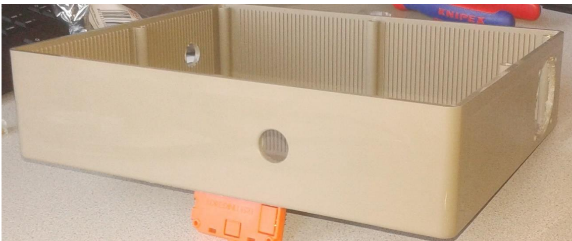
Figure 14: Holes for the cables
