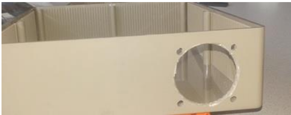
Figure 13: Hole for the socket
