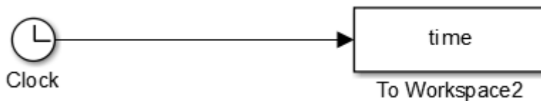
Figure 11: Block use for communication between MATLAB and Simulink to send the values of the variable
