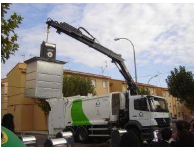
Pic 3. Garbage truck picking up the containers thanks to a crane
