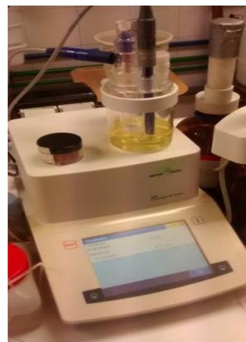
Figura 10.- C20 Coulometric KF Triator de Mettler Toledo
