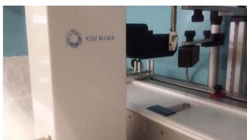
Figura 22. Microscopio BAM (KSV MicroBAM)
