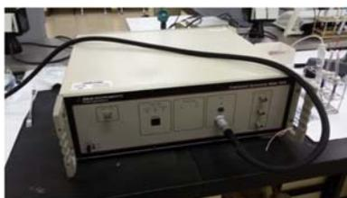
Figura 24. Potenciostato EG&G instruments 263A.
