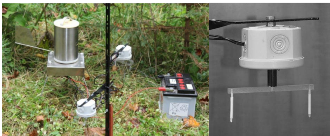
Figure 3. Left: installation of two rotating arm spore traps (centre) and Hirst-type spore trap (left) in SE Czech Republic (Dvořák et al. , 2016). Right: detail of the rotating-arm spore trap (Chandeller et al. , 2014), that is made of two square-section rods covered with double-sided tape.
