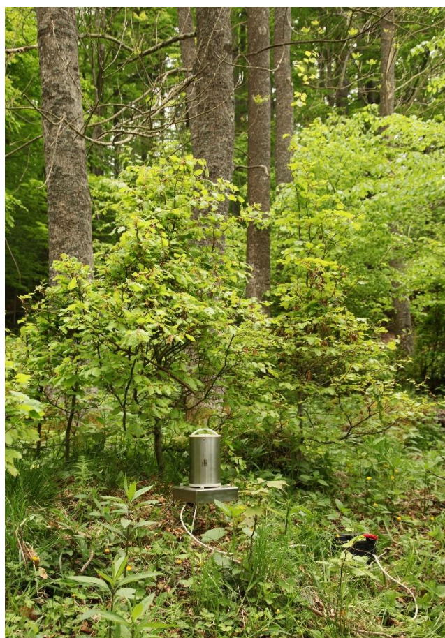
Figure 12. The seven-day automatic volumetric spore trap was placed under the group of moderated-infected ashes in Jelení Hora (Czech Republic), with its orifice 30 cm above soil surface.
