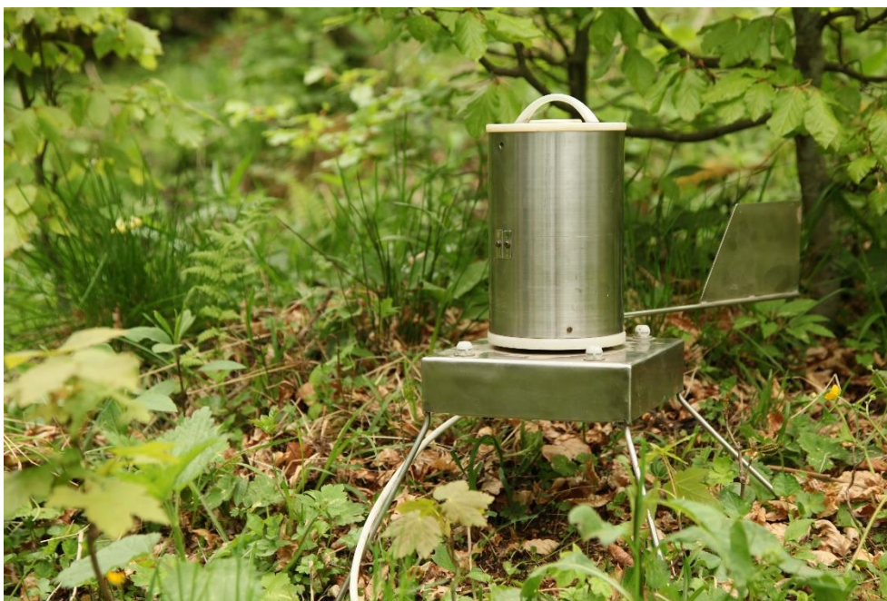
Figure 11. Seven-day automatic volumetric spore trap (SAVST) made by AMET (Velké Bílovice, Czech Republic).
