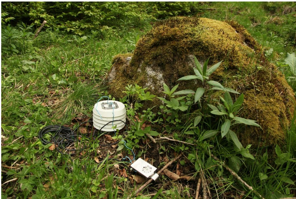
Figure 10. Automatic weather station Signalizátor (Amet, Velké Bílovice, Czech Republic) placed in the assay location.
