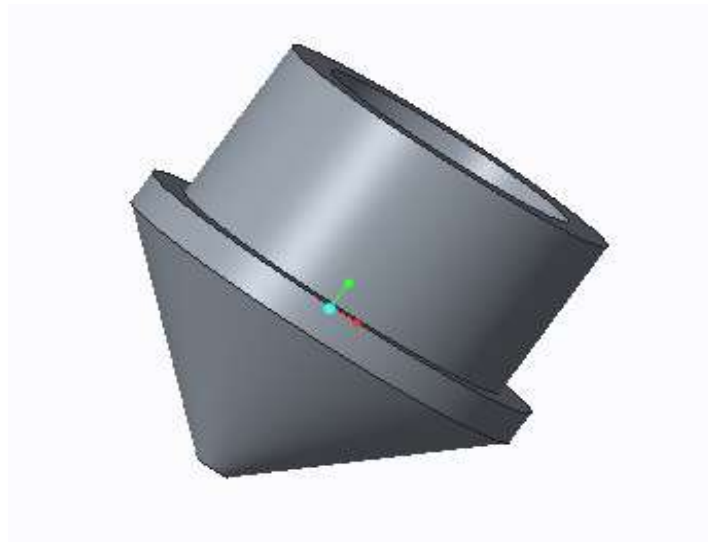
Figure 33. Final shape of the nozzle.
