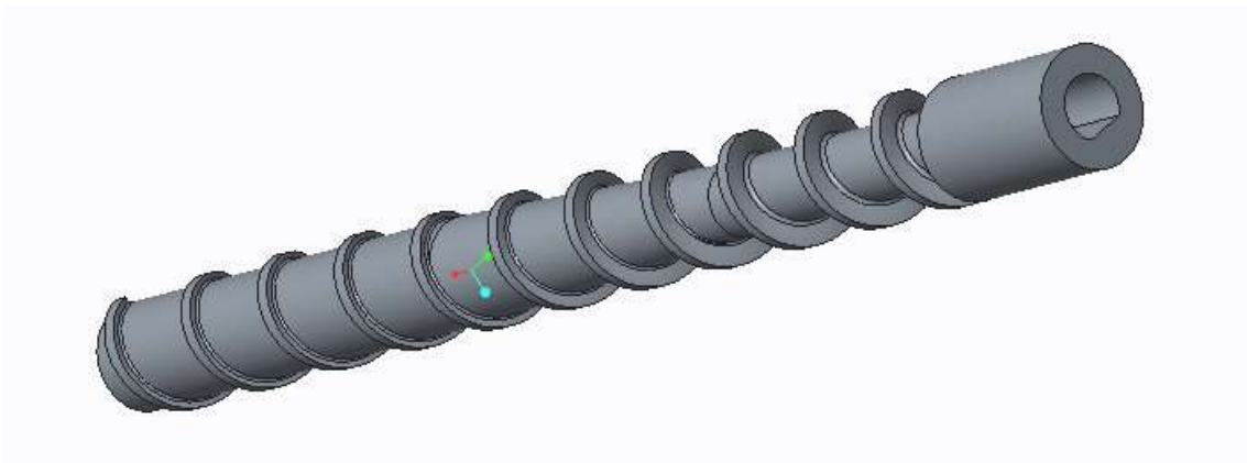
Figure 30. 3D model of the screw. It is visible on it the shape of the connection with the engine.
