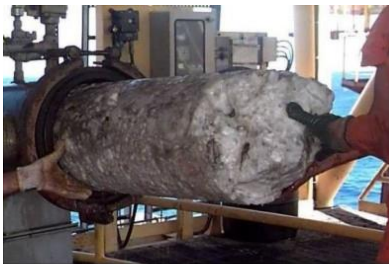
Figure 1.1 Formation of gas hydrate plugged in a subsea pipeline. Picture from Petrobras (Brazil) [3]
