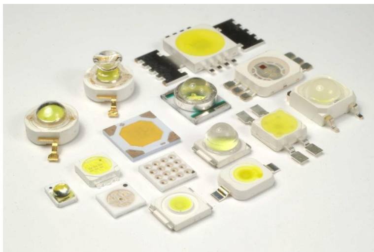
Figura 35. Diferentes tipos de Chips LED. Fuente: http://www.plusopto.co.uk/led-products/high-power.aspx
