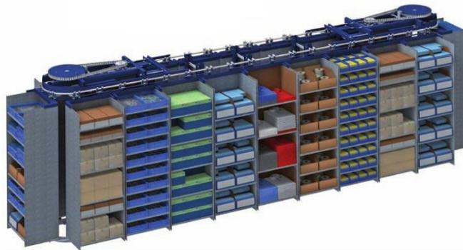
*Figura 4.35- Almacén horizontal spinblock*
