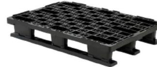
The second most commonly used material is plastic, such as high density polyethylene (HDPE), polypropylene (PP) or polyvinyl chloride (PVC). Their production is more expensive, so their use is internal for the company where they make sure it is not lost or misplaced. This is a more durable and hygienic pallet, it provides higher compression load than the ones made of wood and it can be washed and disinfected without compromising its features.
