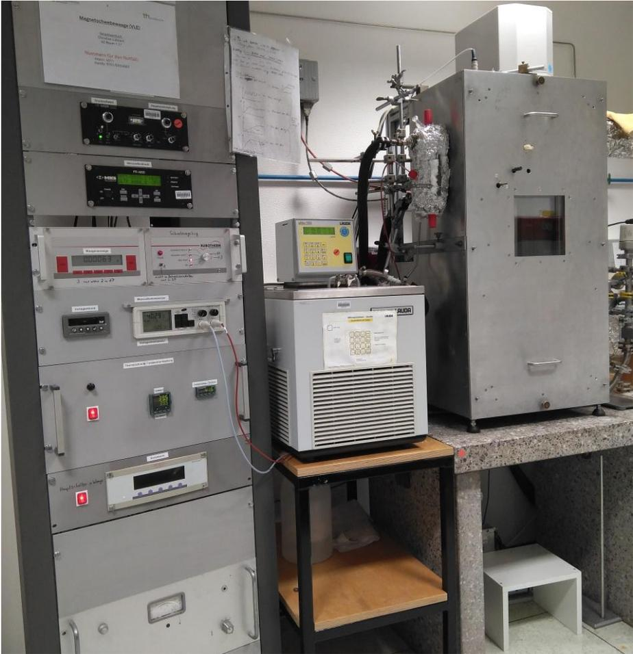
Figure 20. Suspension balance experimental installation
