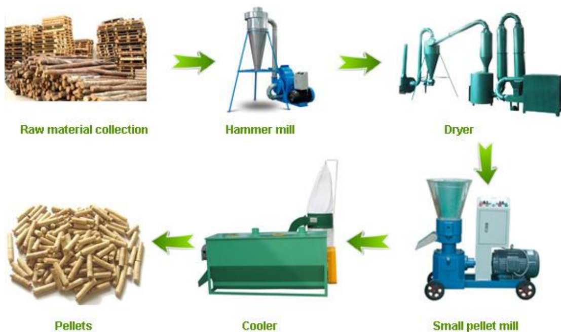
Figure 4.4.15 Process of pelleting.
