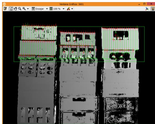
Figure 74: Remarkng the top borders of the containers.
