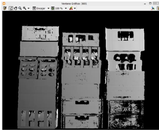
Figure 72: Detecting the containers front surfaces.
