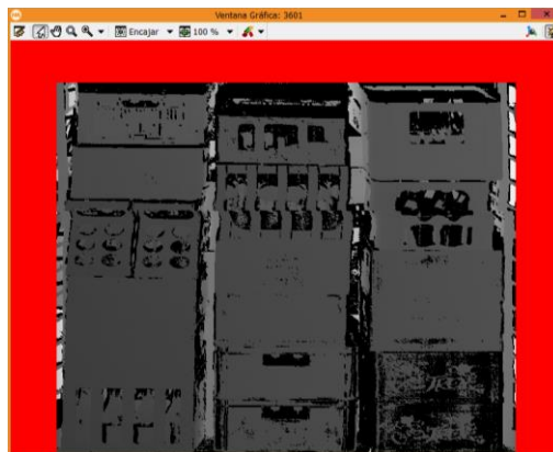
Figure 68: Defining the zones where borders of the rack should be detected.
