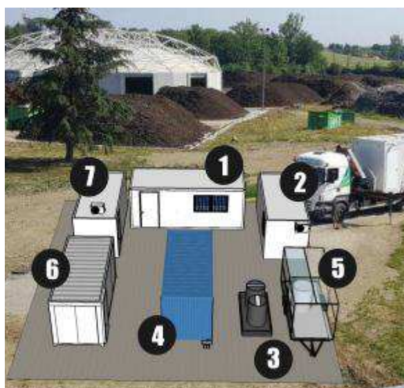
Figure 2 Scheme of the SMS project plant layout: 1. - Working and meeting area 2.- Future urine diversion toilets pilot-scale 3.-Primary settling 4. - Membrane bioreactor 5.- MAD-TAR 6. - Ozonation 7. - Ecotoxicological laboratory
