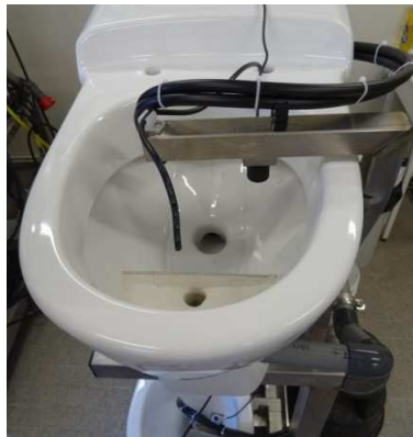
Figure 30 EVAC toilet after change in the geometry of urine compartment
