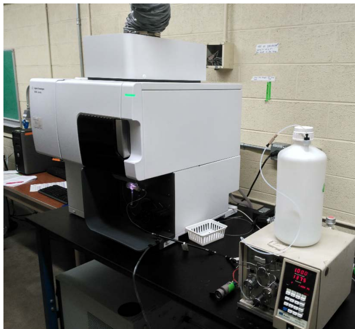
Figure 3.4. HPLC-ICP-OES instrumentation used for Sb speciation.
