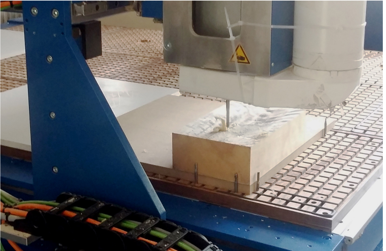
Mould making in CNC milling machine.
