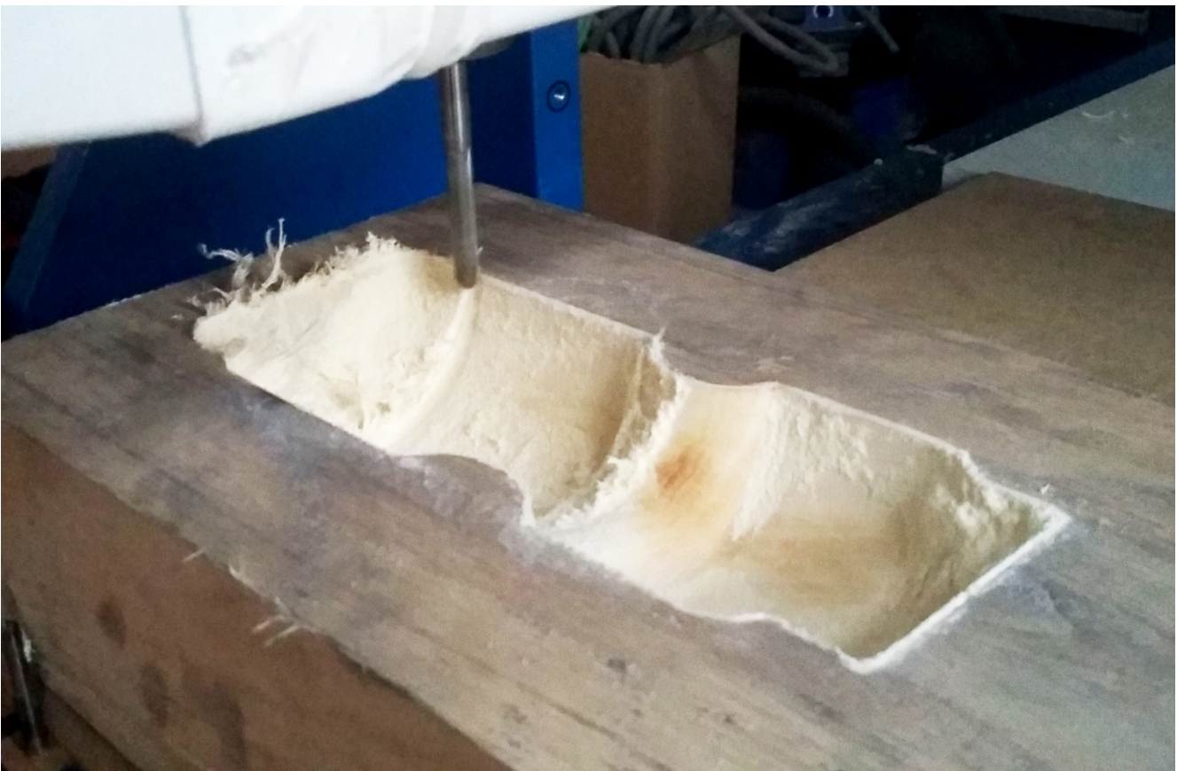
Mould making in CNC milling machine.
