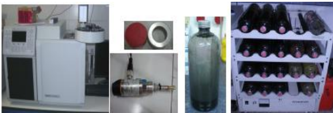
Figure 2: Gas chromatograph, pressure meter, BMP reactor and rotary shaker.
