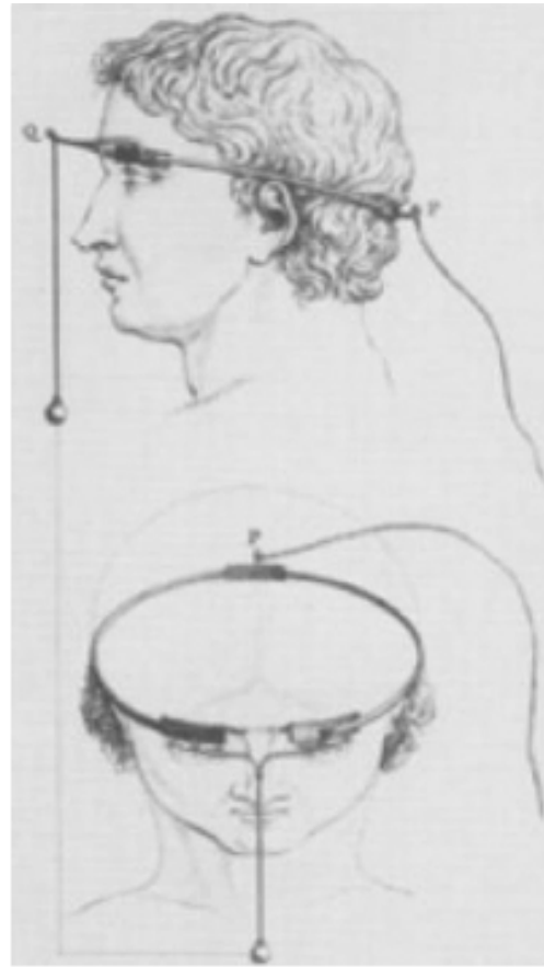
Fig. 2. LeRoy's experimental procedure for ocular stimulation in 1755. A conductive wire was placed around the head of a patient blind from cataract with another one around his leg. The discharge of a Leyden jar passed through the eye of the patient evoking vivid flashes of light.
