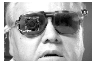
Fig. 7 - A recipient of the Dobbelle implant, first implanted in 1978. In 2000 his external hardware and software was upgraded, including the miniature glasses-mounted camera shown, greatly enhancing the functionality of his prosthesis. Reproduced from (Dobbelle, 2000), with permission.
