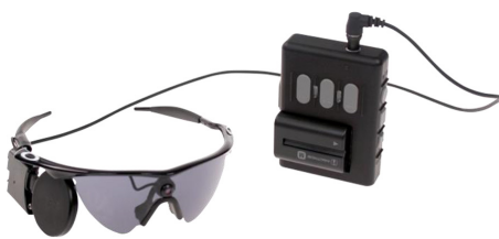
■ FIGURE 1.7 The Argus II Retinal Prosthesis System from Second Sight. (Copyright © 2013 Second Sight Medical Products, Inc. Reprinted with permission.)
