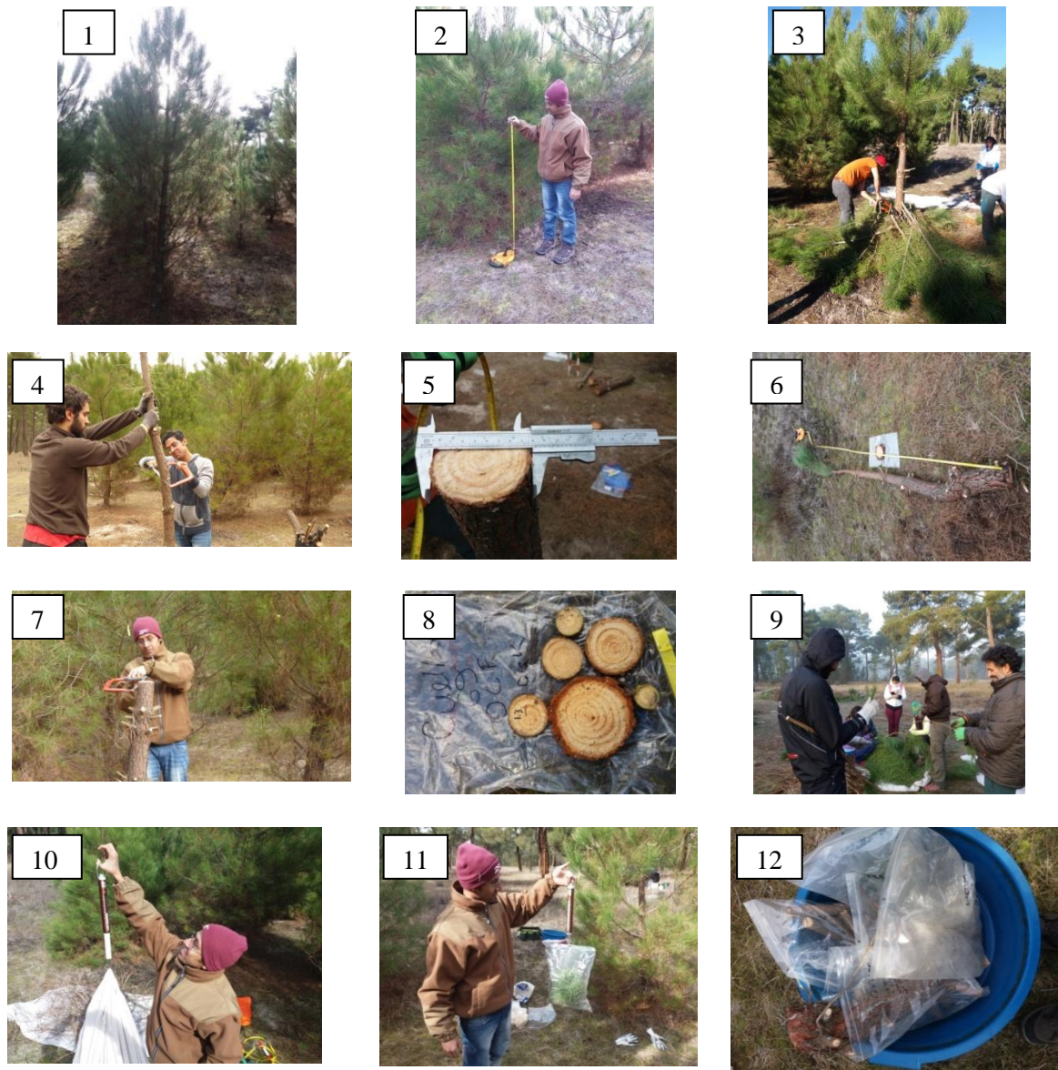
Figure 5: Organization of measurement and sample collection process in experiment plot with different operations. (1), sapling sample in the plot; (2), measurement of ( HMCW; m ); (3), stripping branch from stem; (4) sapling cross-cutting at 1.3 m; (5), measurement of diameter (cm) at breast height (1.30 m); (6), measurement of total height ( ht; m ); (7), cross-cutting into stem and disks; (8), disk samples; (9), stripping of needles from branches; (10), weighting totals fresh mass of stem, branch, and needle; (11), weighting sample; (12), collected samples under tree to avoid moisture content loss in the field (Photo Credit: Pavel, M.A.A., Sara. U. P, Cristóbal, O. A. and Brenda, I. M. R.).
