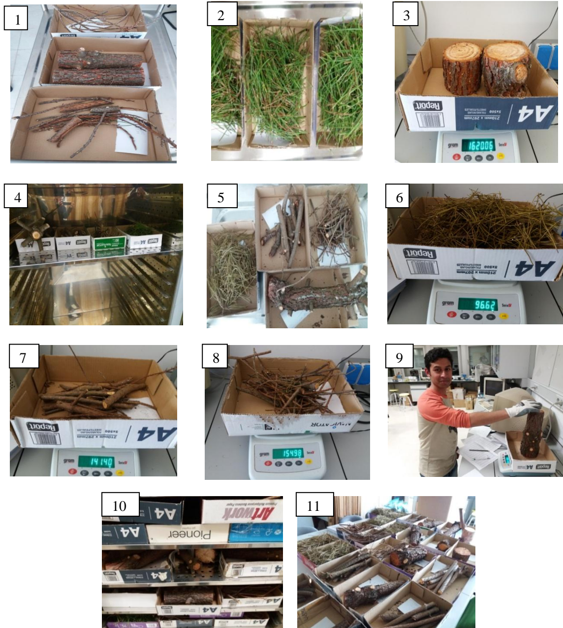
Figure 7: Weighting and dry procedure for samples on arrival at the laboratory, (1), fresh sample of stem, branch in a paper box; (2), fresh sample of needle in a paper box; (3), fresh sample weighting; (4), drying in the oven; (5), dry sample of stem, branch and needle for weighting again; (6), weighting of the dry needle sample; (7), weighting of the dry branch (2-7cm) sample; (8), weighting of the dry branch (2cm) sample; (9), weighting of the dry stem sample; (10), again sample put in the oven for drying; (12), keep out the final dry sample from oven (Photo Credit: Pavel, M.A.A. and Cristóbal, O. A. ).
