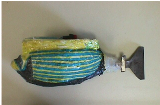
Figure 6. A robotic fish equipped with a single IPMC tail fin [9].
