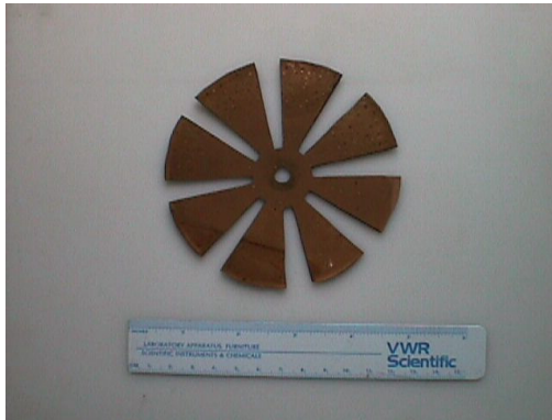
An eight finger synthetic muscle. It has a thickness of approximately 2 mm.
