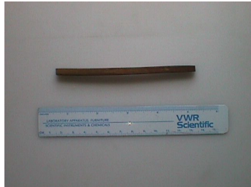
A rod shape synthetic muscle. It has a rectangular cross-section of approximately 8 mm x 8 mm.
