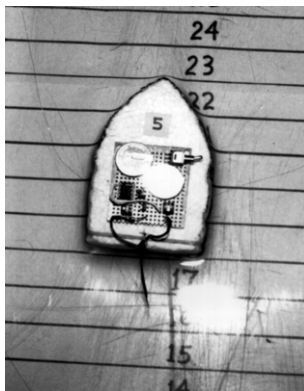
Figure 4. Robotic swimming structure (top) and swimmer with muscle (bottom). The scale shown is in cm [9].
