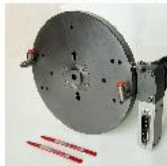
Rotating table for 2 shot applications
