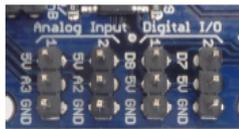
*Fig.1 – Digital and Analog ports*
