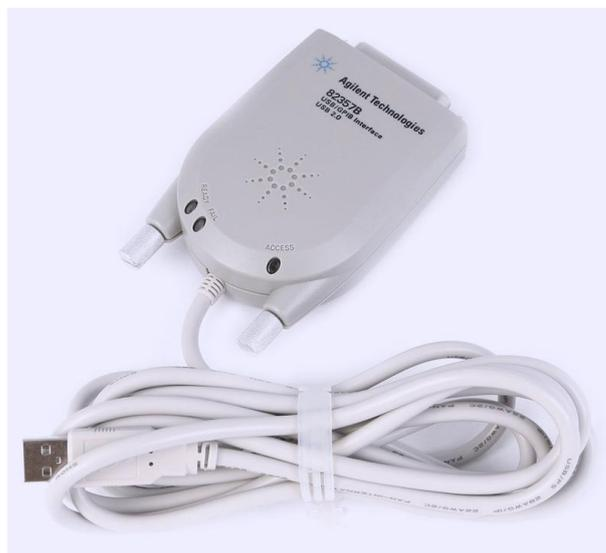
**Figura 3.13.** Cable GPIB/USB.
