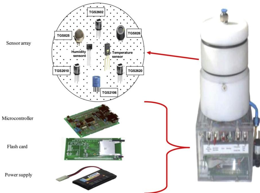
Fig. 2. Portable electronic nose (Fuchs, Strobel, Siadat, & Lumbreras, 2008).
