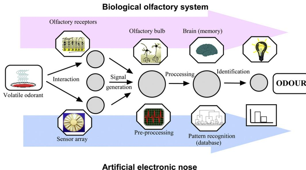
Fig. 1. Analogy between the biological and the electronic noses.
