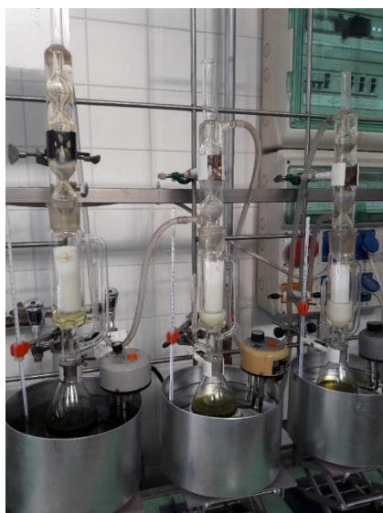
Figure 12. Last stage of the Soxhlet extraction.
