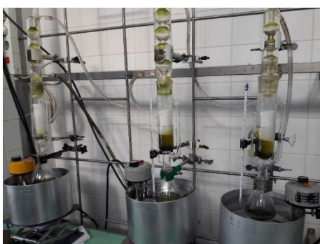
Figure 11. First stage of the Soxhlet extraction.
