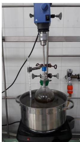
Figure 13. Stirred tank extraction.
