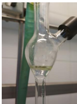
Figure 15. Essential oil on the top of water in Clevenger distillation unit.
