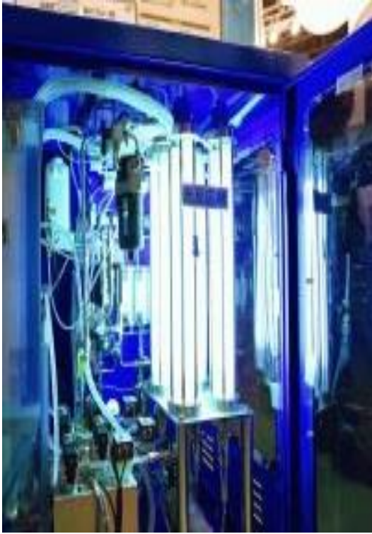
Figure 13: Photocatalytic water purification system [21]
