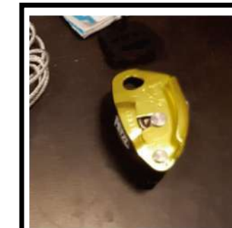
Self-braking descender from Petzl, only made for right-handed people.
