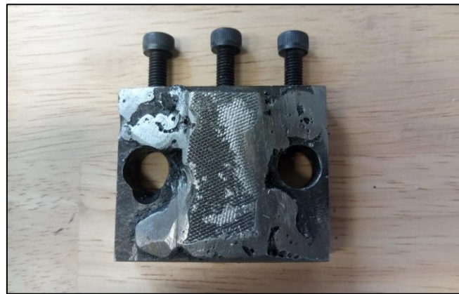
Damaged gripping surface
