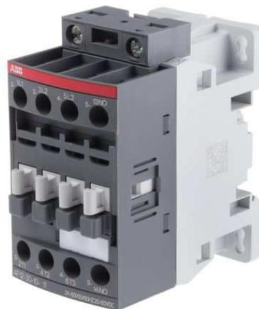
**Fig. 14.-** Contactor ABB AF12-30-10-11 de 28 A, 3NA, bobina de 24 Vac, gama AF de RS-ONLINE.
