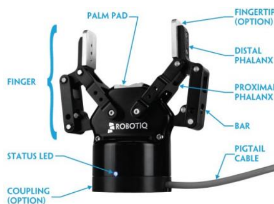
Figure 17. Two-finger gripper ( Robotiq 2F-85, Instruction manual )
