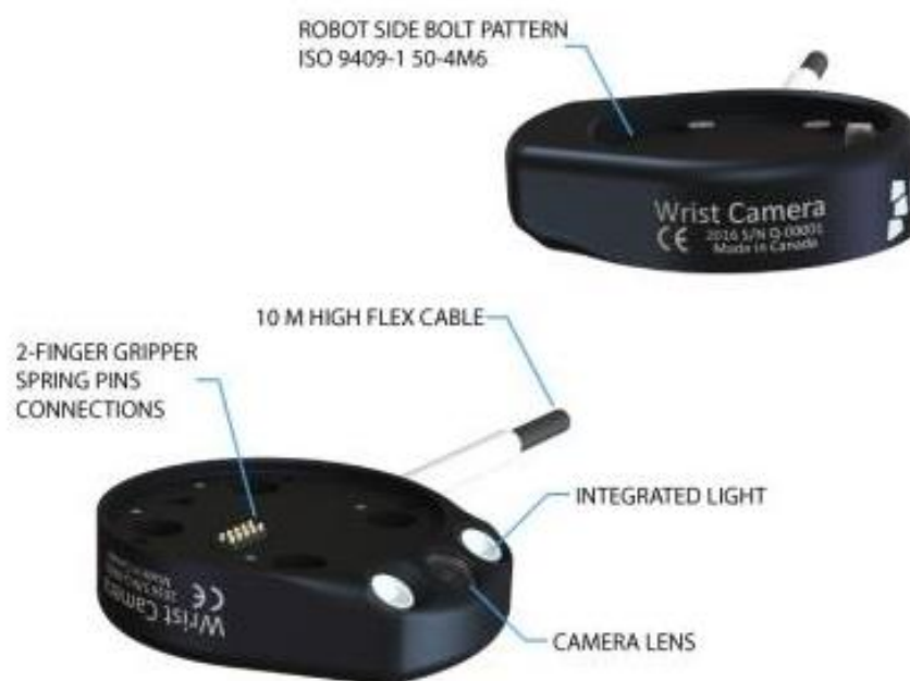
Figure 27. Main features of Wrist Camera. (RobotiQ. (n.d.). Wrist Camera Instruction Manual )
