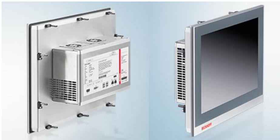
Figure 7- PLC and Touch Panel CP2215-0020
