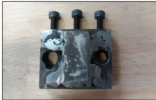
Damaged gripping surface
