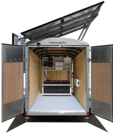
Figure 13. Example 5. MS-225 SOLAR GENERATOR – Mobile Solar
