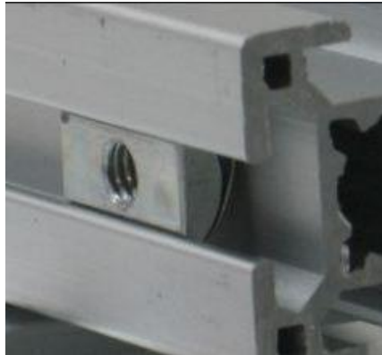
Figure 48. Detail of the T-Nuts in the beams.
