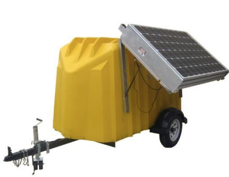
Figure 8. Example 1. Solar Trailer Folded
