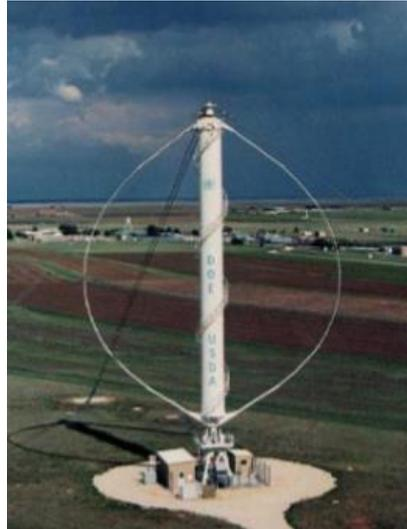
Figure 4.5.-Vertical axis turbine[6]
