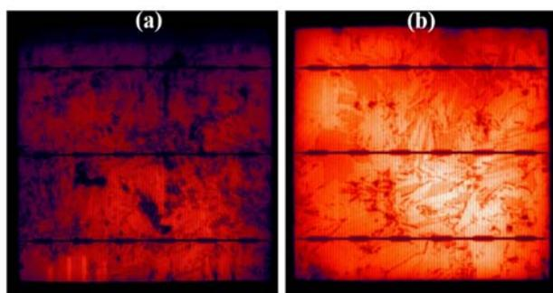
**Figure 2.** PL images of solar cells with efficiencies of 16.4% (a) and 17.4% (b) (average efficiencies). LUT contrast is the same in both images.
